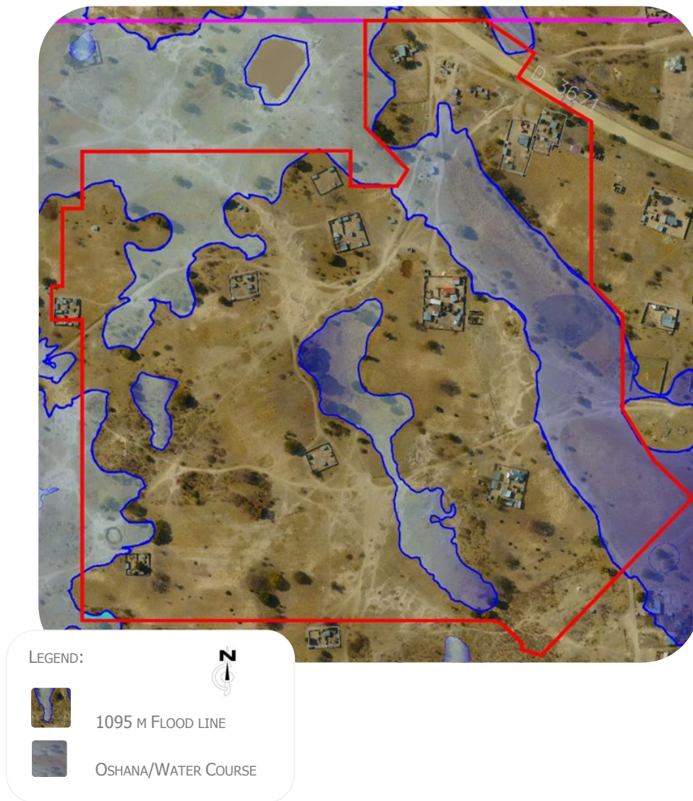
Figure 7: 1095 m Flood line on the site
