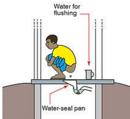
Design of squatting pan with water seal, pour flush system. ( https://en.wikipedia.org/wiki/Pit_latrine )
