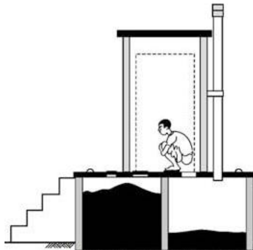
Elevated double vault pit latrine. This model can be used in flood prone areas or where groundwater is close to the surface.
