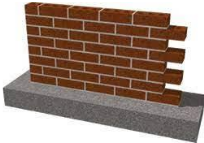
Figure 10: Tothing in a wall to continue construction at a later date (tothing in wall construction - Google Search)
