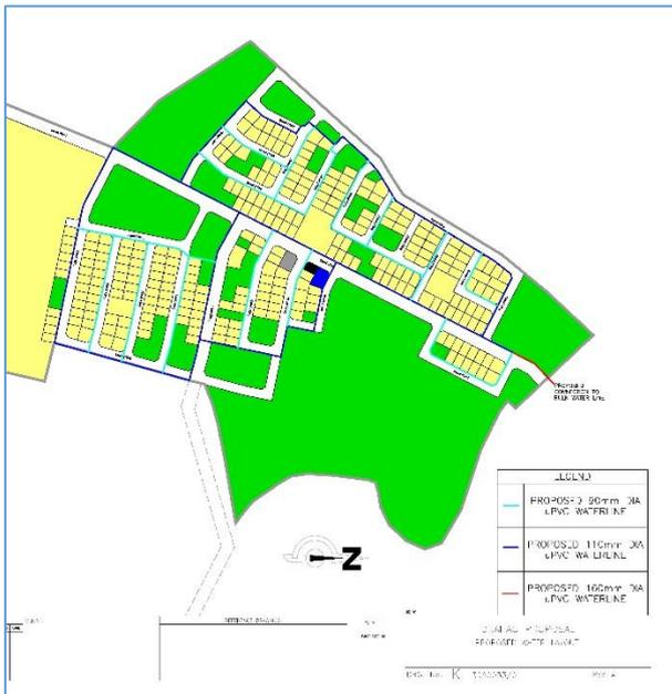
Layout displaying the preliminary design of water reticulation in the project area.
